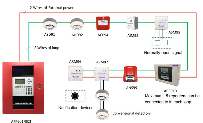
Maximum 30 conventional detectors can be connected to in each zone.
